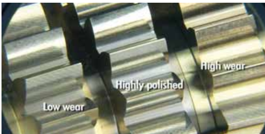
Figure 4: Gears showing increasing wear.
