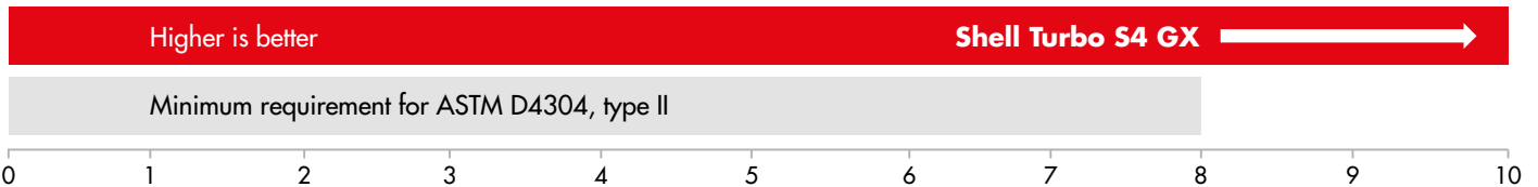
Figure 3: FZG performance of Shell Turbo S4 GX against the ASTM D4303 type II requirements.
