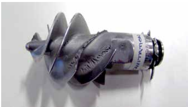
FIGURE 1: Erosion damage to a pump.
